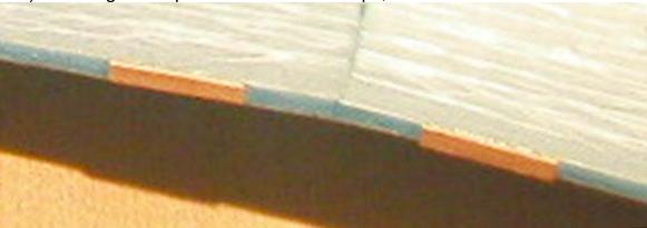
c) Glue them to the front and rear of the upper and lower wings where the rubberbands will cross the wings. Press them in until they are almost flush with the leading edge of the wing, or you might need to sand the fuselage a little to make the wings fit on.
