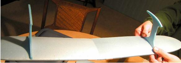
g) Glue the Wing Struts to the bottom wing 9" from the center.
