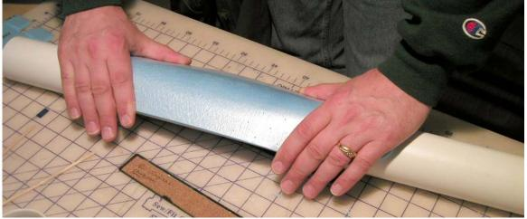
Now the wing pieces probably have more curve than they need. Grab one of the parts with the airfoil shape, (Like the struts, or the landing gear mounts, although the fuselage will do too.) and use it to check your airfoil. If it's not an exact fit, massage the wing a little until it's pretty close. The glue will do the rest.
